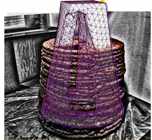
Left: A model by MArch student Rudi Vermeer of a seed cultivation centre in Pretoria, 2017. (Photograph by Mostert van Schoor). Right: A 3-D printed earth column/formwork by March: Arch Tech student Asher de Jager, 2023.
